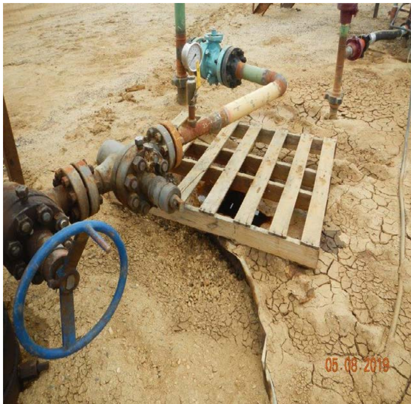
Photo#2: Peters 0781 9-13H12 API# 057-06584. Pallet covering what Operator identified as mouse hole.
