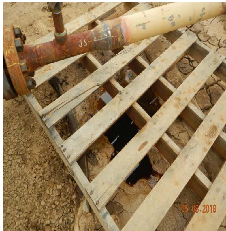
Photo#3: Close up of mouse hole showing overflow of oily waste.
