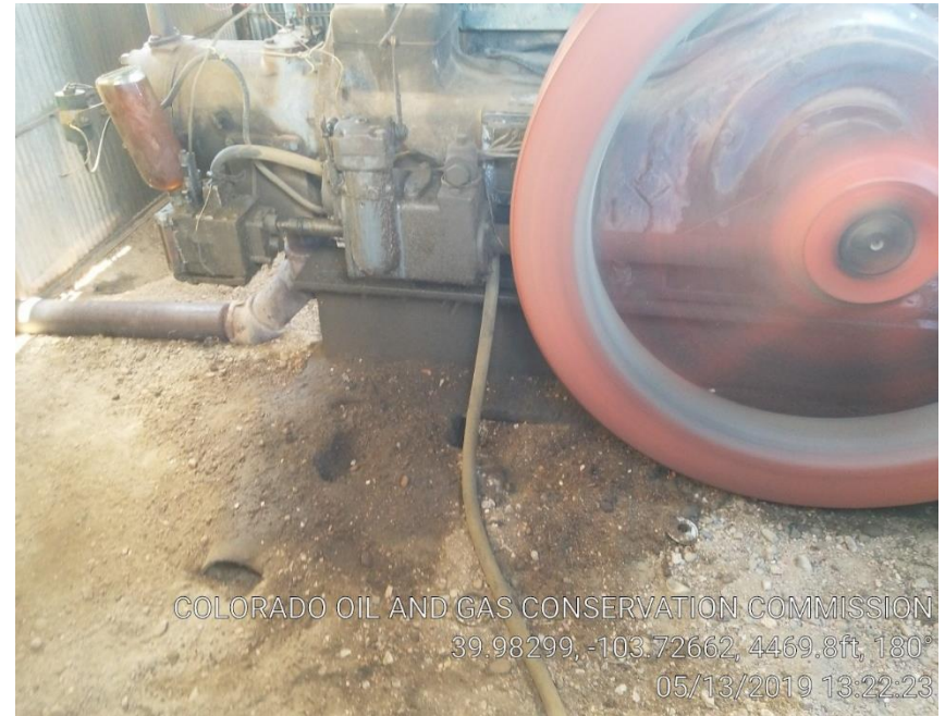
Pic 14 stained soil inside motor house
