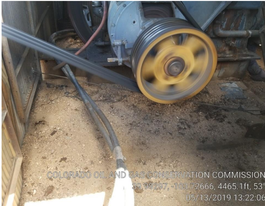
Pic 13 stained soil inside motor house
