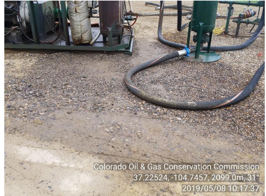
PHOTO 4: THERE IS AN AREA APPROXIMATELY 7' CIRCLE OF IMPACTED SOIL LEADING FROM THE SOUTHWEST CORNER OF COMPRESSOR SKID. Non E&P Waste not properly stored, handled, transported, treated, or disposed per Rule 907A. Contact COGCC EPS staff. CA DATE 6/8/19
