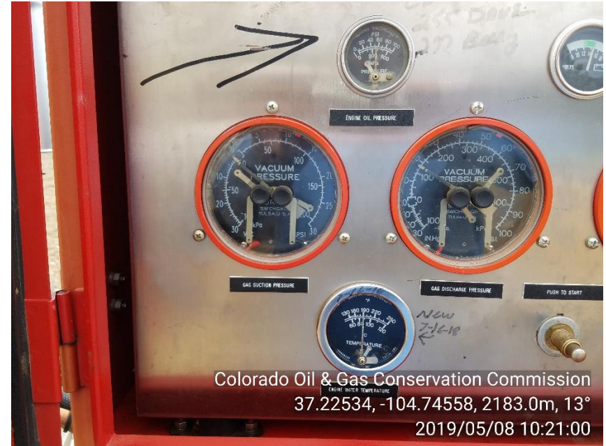
PHOTO 5: WELL APPEARS TO BE ON A VACUUM. Provide COGCC with documentation showing approval of use of vacuum pump. CA DATE 5/23/19
