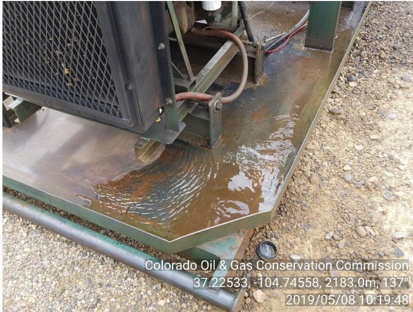
PHOTO 3: OIL SHEEN ON WATER IN COMPRESSOR SKID CONTAINMENT THERE IS ALSO IMPACTED SOIL ALONG THE WEST EDGE OF COMPRESSOR SKID. Securely fasten all valves, pipes, and fittings to ensure good mechanical condition, inspect at regular intervals and maintain in good mechanical condition per Rule 605.d. CA DATE 6/8/19
