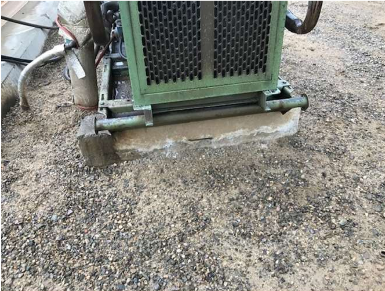
PHOTO 1: THE IMPACTED SOIL AROUND THE ENGINE SKID WAS REMOVED FROM THE LOCATION. (PHOTO TAKEN DURING RAIN SHOWERS).
