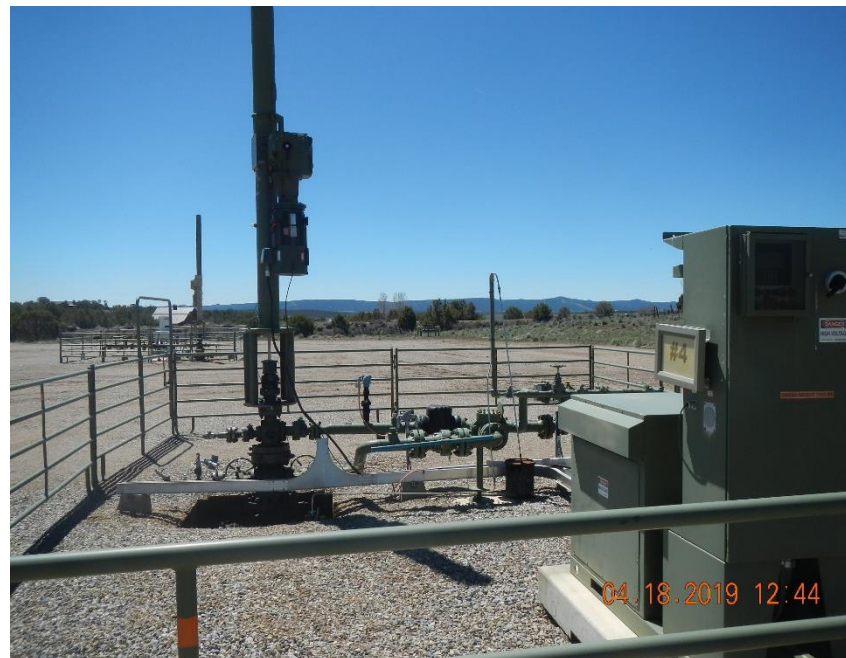
Linear rod pumps on both wellheads.
