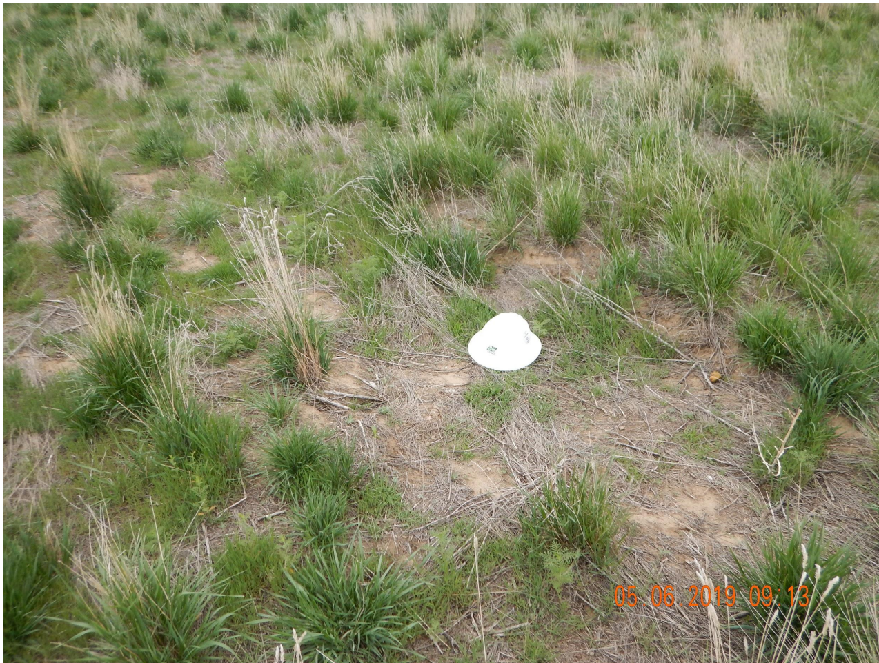
Photo 4. Photo taken from the well location. Photo illustrates subsidence at the wellhead and vegetation around the wellhead is not reflective of reference area vegetation.
