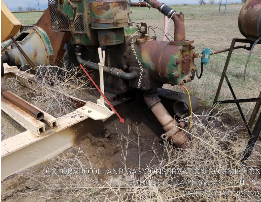
Pic 5 stained soil by motor
