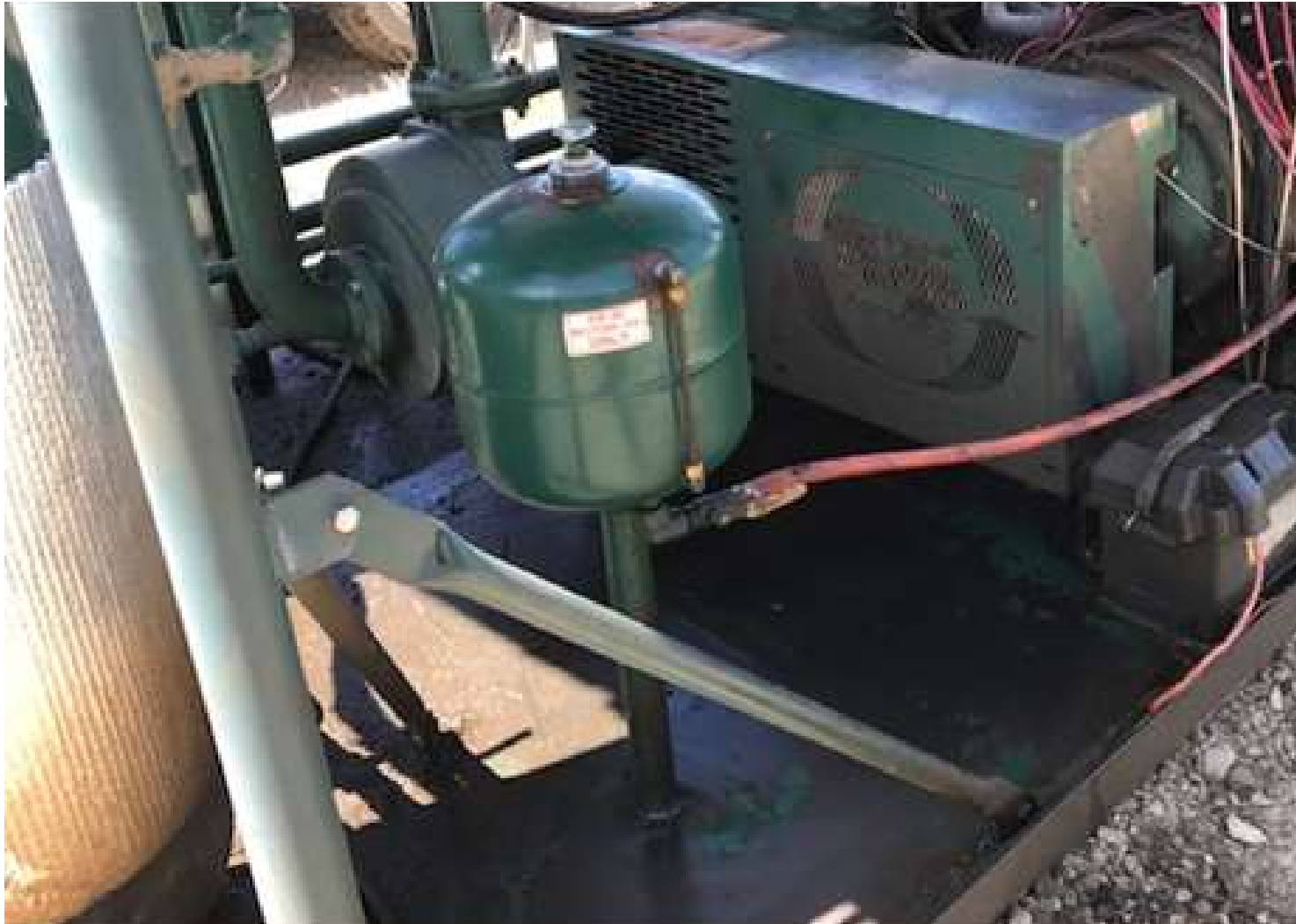
PHOTO 5: THE ABSORBENT PADS AND OIL ACCUMULATION WERE REMOVED FROM THE LIQUID RING SKID AND CLEANED UP.
