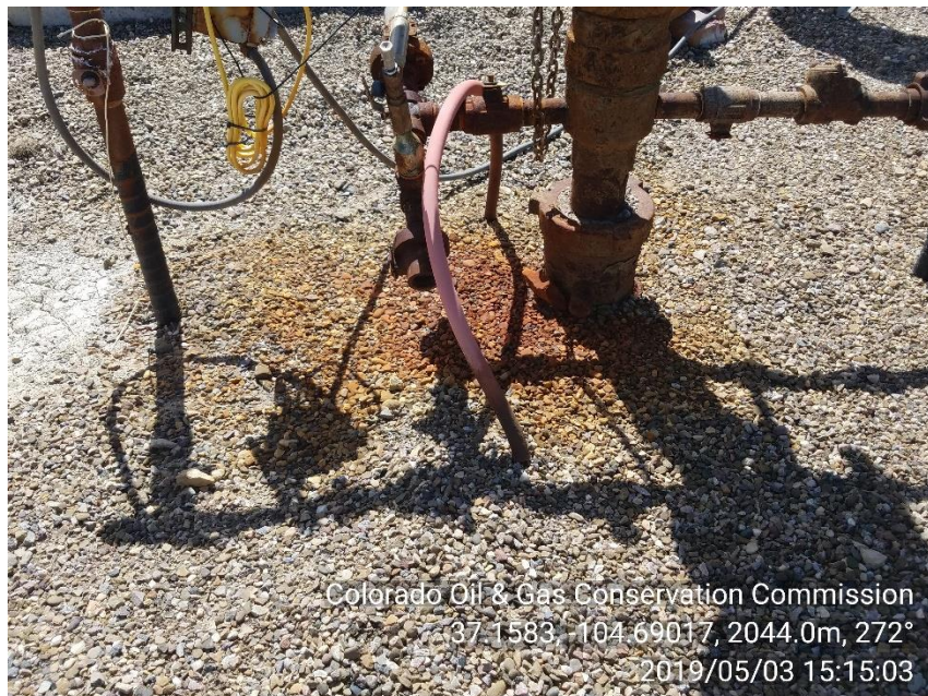
PHOTO 3: RUST COLORED IMPACTED SOIL APPROXIMATELY 4' BY 3' AREA AROUND WELLHEAD
