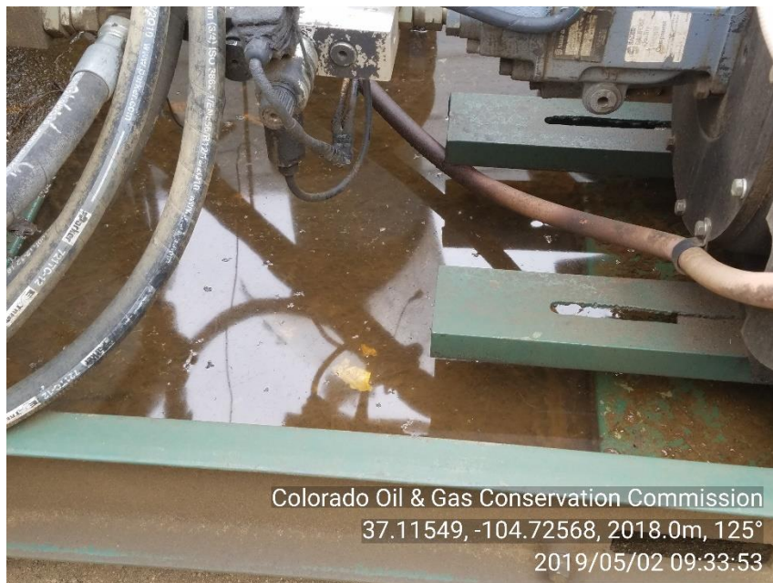
PHOTO 3: APPROXIMATELY 2" TO 3"S OF STANDING OILY WATER IN PRIME MOVER ENGINE SKID.
