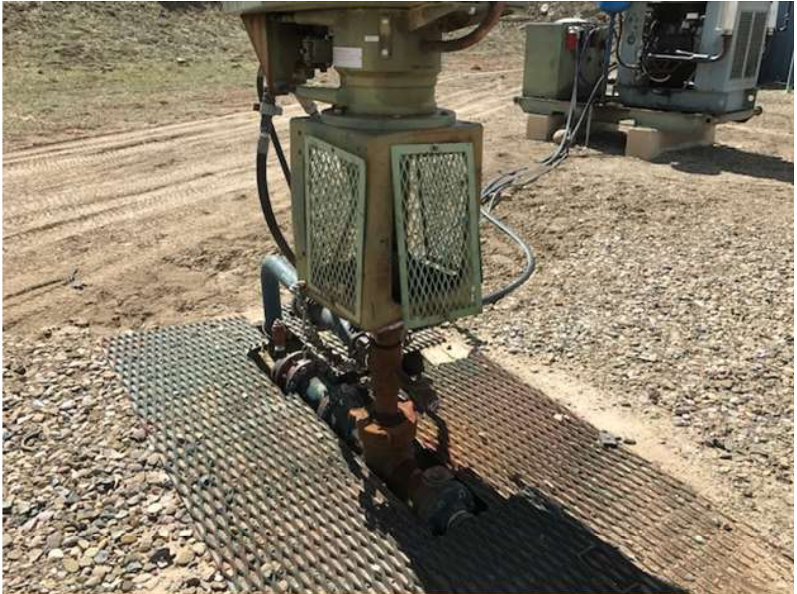
PHOTO 4: REPLACED THE PACKING TO ELIMINATE THE WATER LEAK. PACKINGS ARE SECURELY FASTENED IN COMPLIANCE WITH RULE 605.D.
