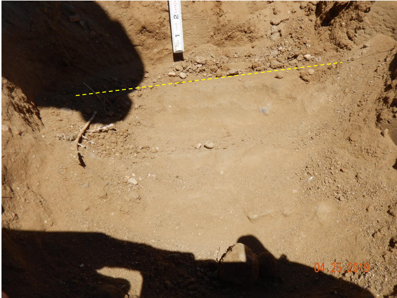
Photo 12: Continued from photo 11. Photo shows compaction concerns beginning 7 inches below ground level.
