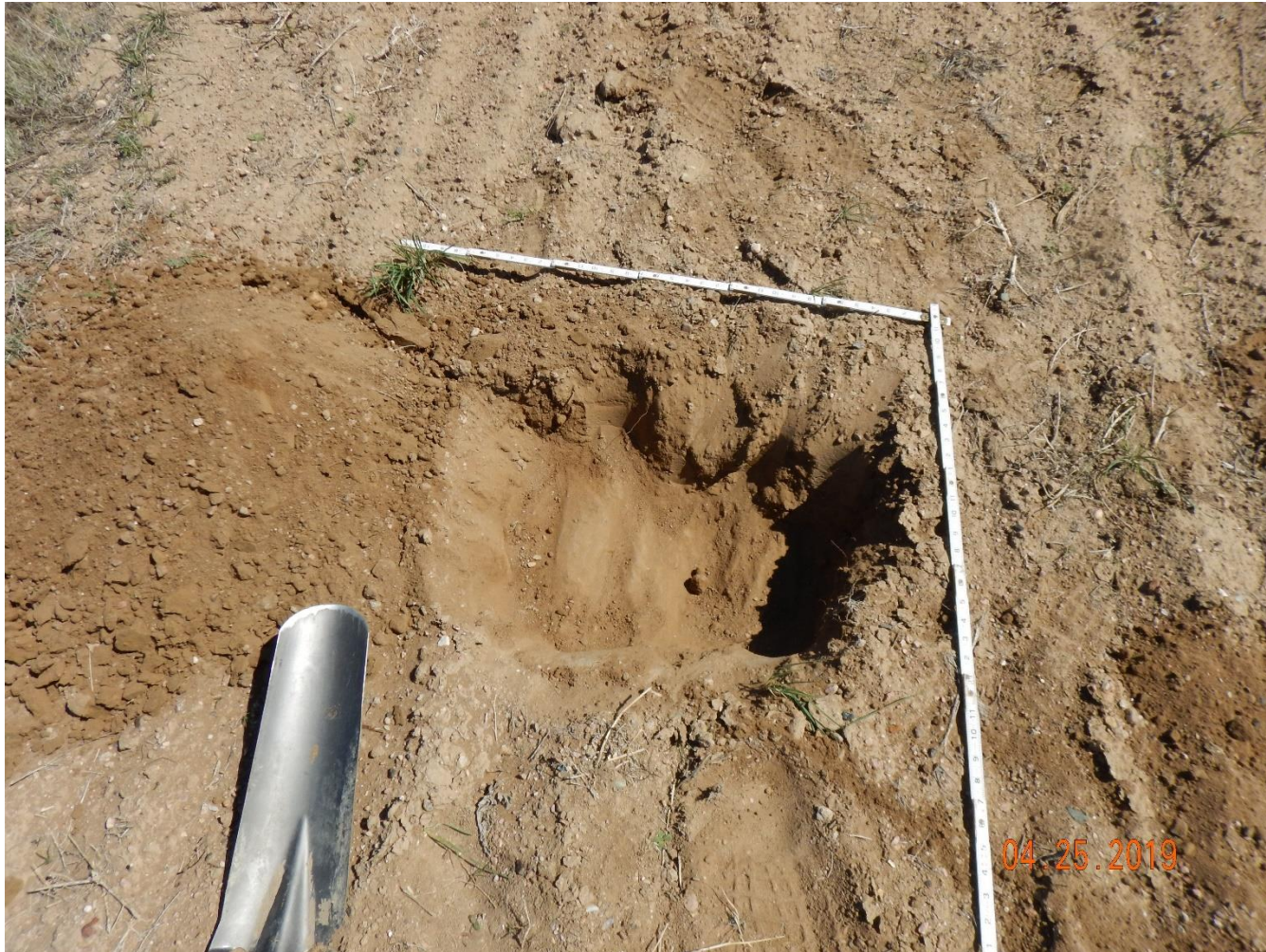
Photo 11: Photo taken from the access road. Photo shows inspector dug a pit to test for compaction alleviation at access road. Inspector was able to find multiple zones of compaction starting at 7 inches below ground level.
