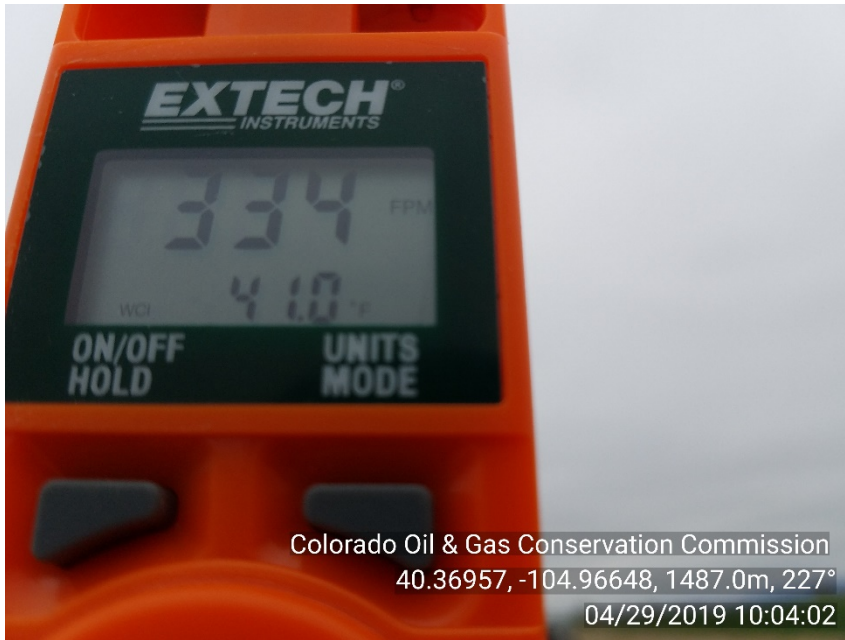
Anemometer (3.79 MPH)
