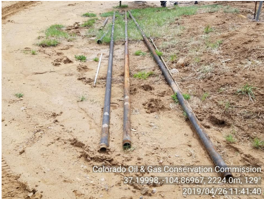
PHOTO 3: UNUSED EQUIPMENT STORED ON LOCATION. 3 JTS TBG, 1 SUB, 1 DOWNHOLE PUMP, 1 STATER AND 1 JT ROD.
