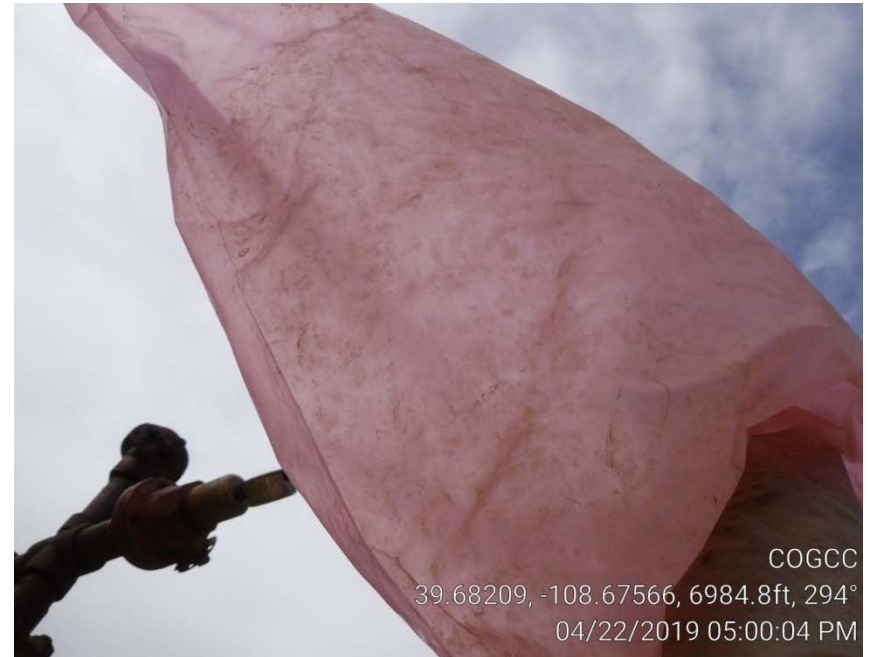
Photo 4. Gas rate measured with 3 cubic ft bag.
