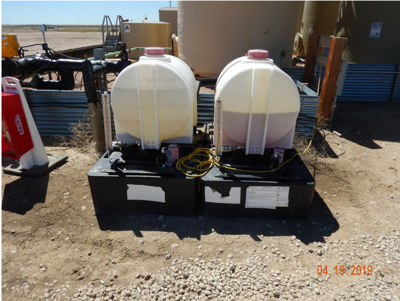
Photo 15: Photo shows secondary containment BMPs in proper functioning condition.
