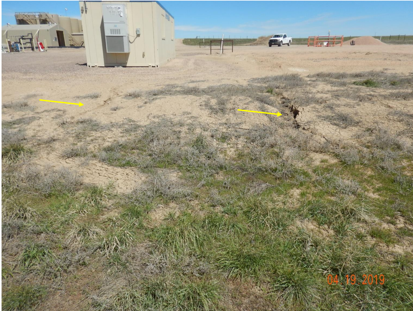
Photo 7: Photo shows stormwater erosion degradation on location/interim areas.
