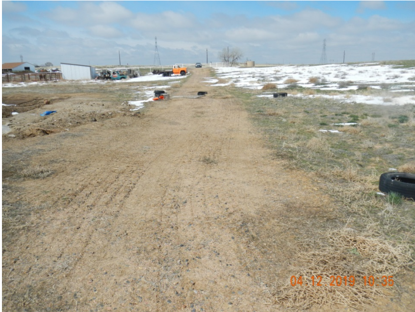
Photo 1. Photo taken from the access road, facing West. Appears Operator has performed final reclamation activities at the location with evidence of drilling rows. However along the access road the reclamation is not at percent cover and has non-uniform establishment of vegetation cover.
