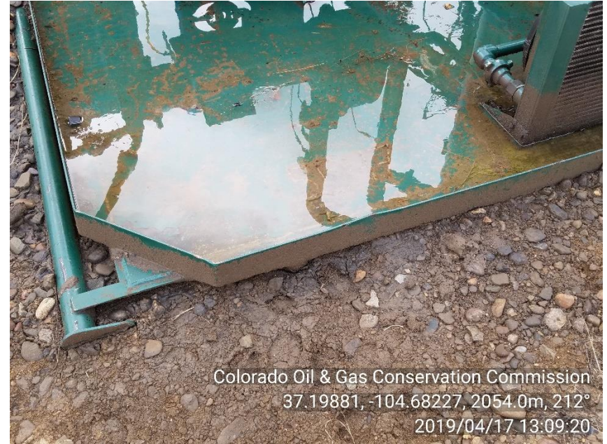
PHOTO 8: APP. 2" OF STANDING WATER WITH OIL CONTAMINATION IN COMPRESSOR SKID IS WITHIN APP. 2" FROM RUNNING OVER
