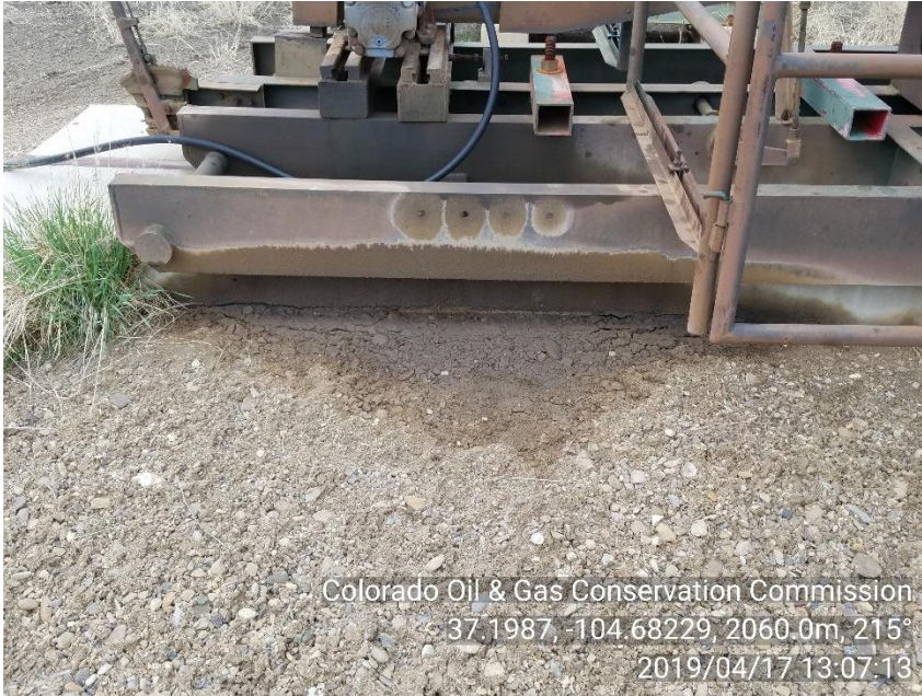
PHOTO 7: IMPACTED SOIL ON NORTH SIDE OF PUMPJACK HYDRAULIC MOTOR.
