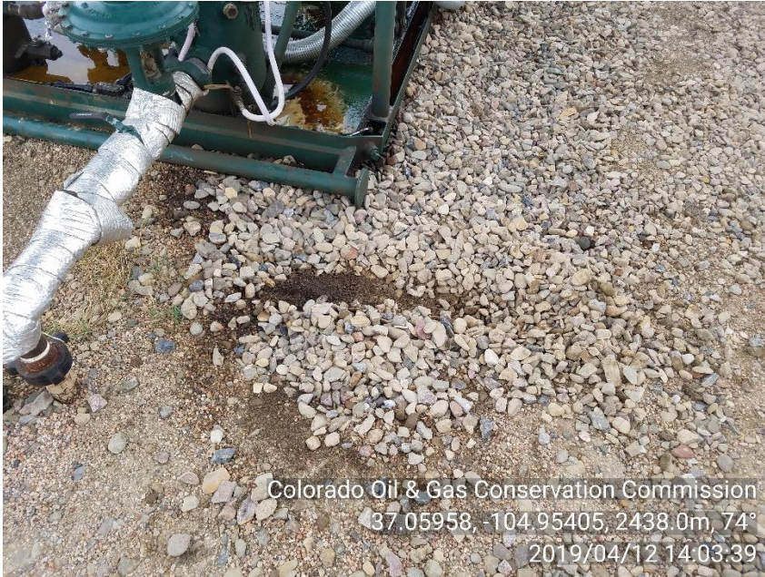
PHOTO 3: IT APPEARS THAT THERE WAS AN ATTEMPT TO REMOVE SOME IMPACTED SOIL IN THE NEAR PAST AS THERE IS SOIL REMOVED FROM THE SOUTH SIDE OF COMPRESSOR SKID BUT AS SHOWN IN THIS PHOTO SOME OF THE IMPACTED SOIL WAS NOT REMOVED AND WAS COVERED UP WITH CLEAN GRAVEL.
