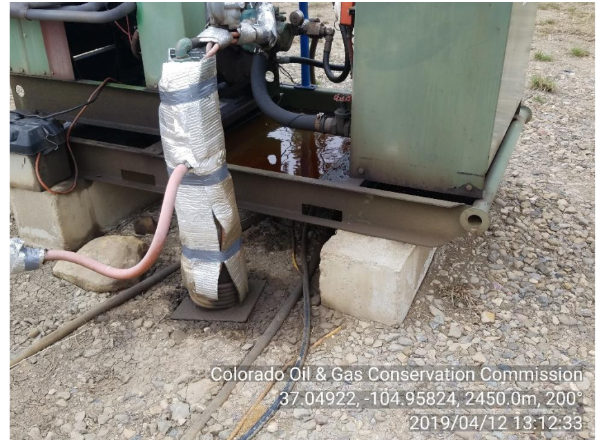
PHOTO 4: THERE IS APP. 2' AREA ON IMPACTED SOIL AROUND BASE OF FUEL GAS SEPARATOR ON PRIME MOVER ENGINE SKID. ENGINE SKID HAS APP. 1' STANDING OIL IN SKID CONTAINMENT.
