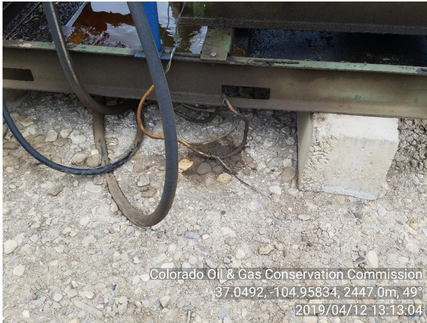
PHOTO 5: APP. A 8" ROUND AREA OF IMPACTED SOIL ON WEST END OF PRIME MOVER ENGINE SKID.
