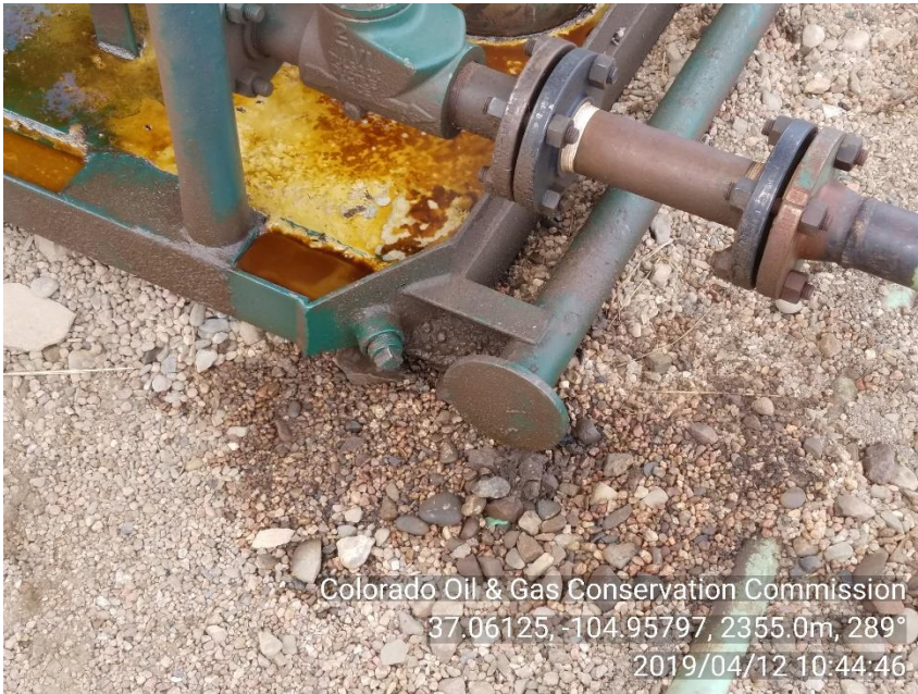
PHOTO 3: SECONDARY CONTAINMENT ON COMPRESSOR SKID IS FULL OF OIL & WATER AND IS RUNNING ONTO LOCATON.
