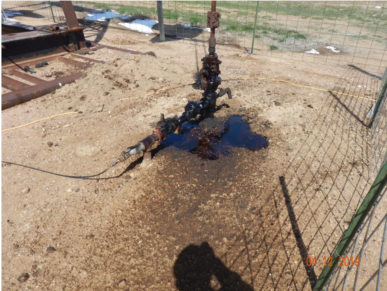
Photo 6: Photo taken from the well. Photo shows chemicals/fluids are being discharged from the well. Photo also shows contaminated soils.
