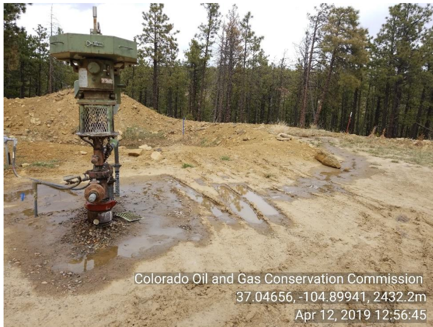
Photo 3 Packing on well head appears to be leaking and traveling down location
