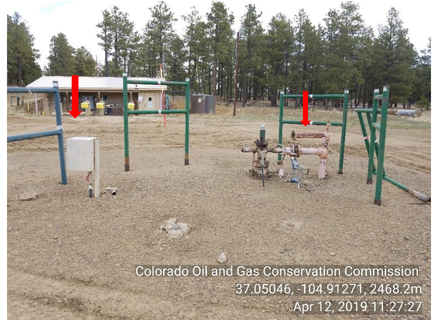
Photo 4 HR#29-14V WH. Unused, unmarked and not LOTO risers.
