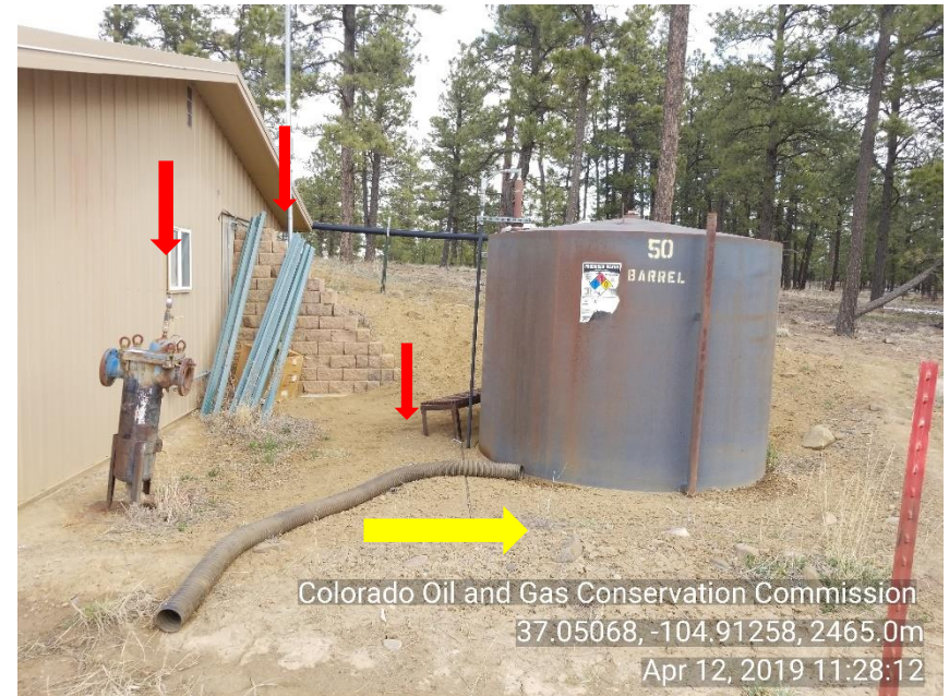
Photo 6 Unused equipment Filter pot, hose and metal. Inadequate berm around tank.
