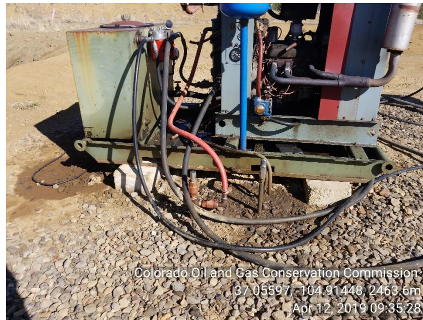
Photo 4 Stained soil around HYD motor skid
