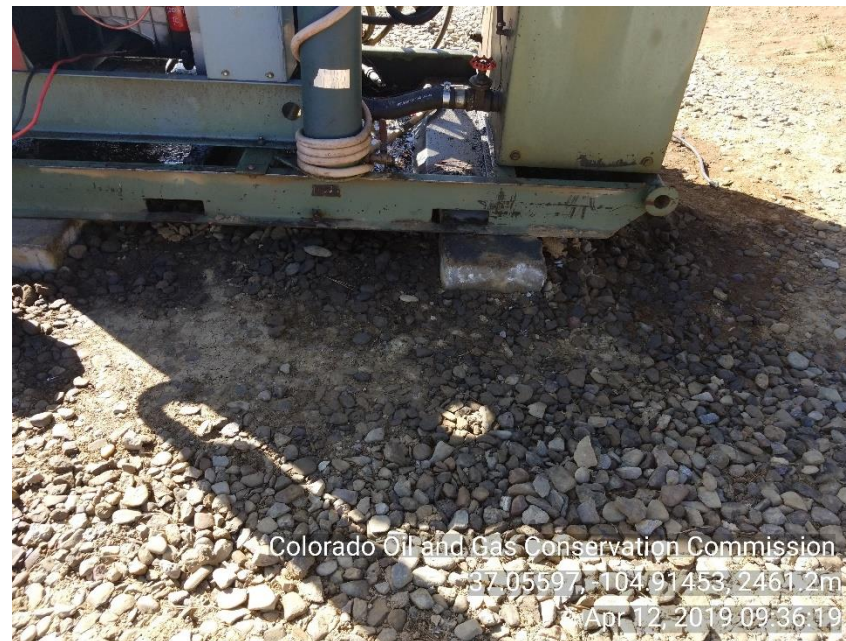
Photo 6 Stained soil around HYD motor skid
