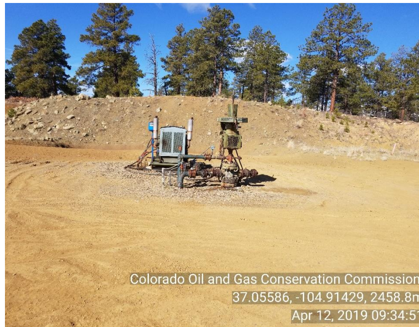
Photo 2 WH and HYD motor skid
