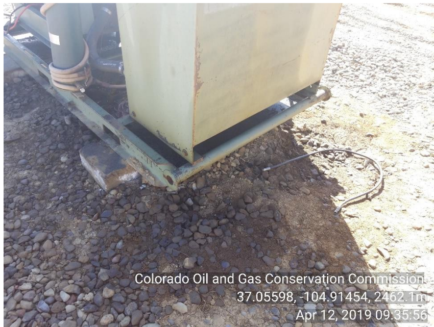
Photo 5 Stained soil around HYD motor skid
