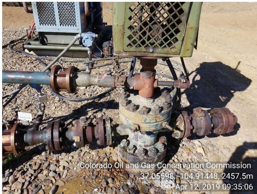
Photo 3 Packing leaking at time of inspection
