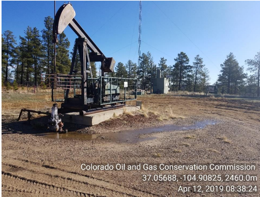
Photo 3 PU. Packing appears to be leaking fluid has travel approximately 20ft on location.
