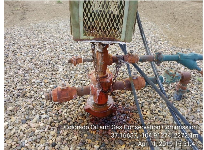
Photo 4 Mechanical issue packing leaking. Stained soil around WH
