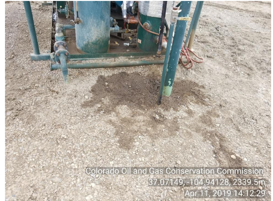
Photo 6 Stained soil around Liquid ring
