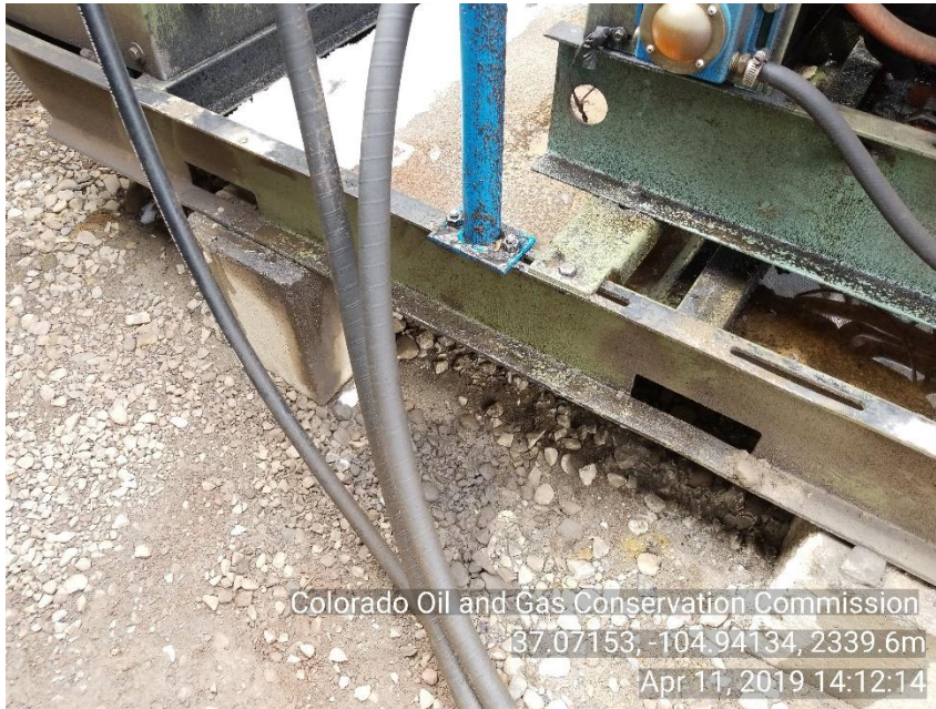
Photo 5 Stained soil around HYD skid
