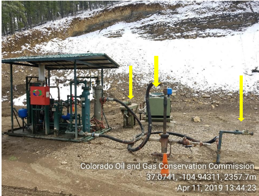
Photo 3 Liquid ring skid. Unused equipment (HYD skid, PC Drive). Unused, unmarked and not LOTO riser.
