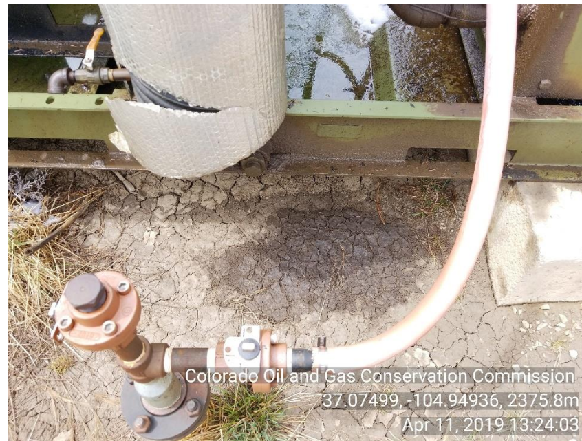
Photo 3 stained soil around HYD skid
