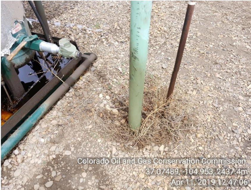
Photo 3 Stained soil around liquid ring riser
