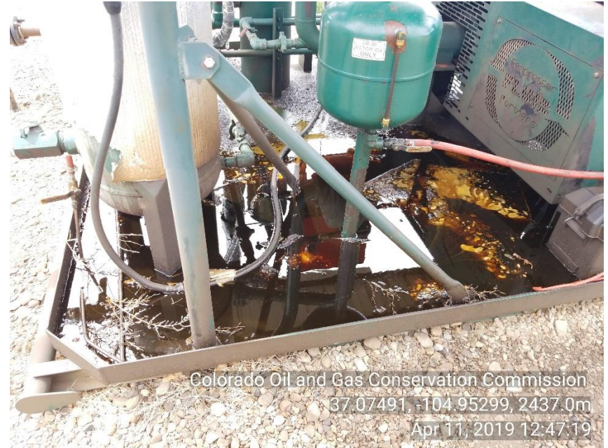
Photo 4 Liquid ring skid almost full possible storm water issue.
