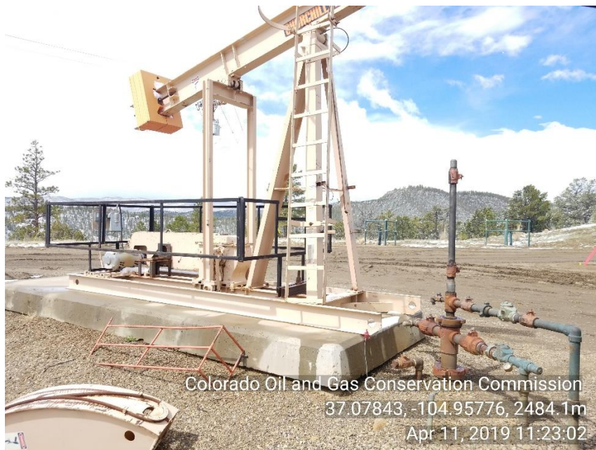
Photo 3 Unused equipment; PU, Cement base, horses head and guard.
