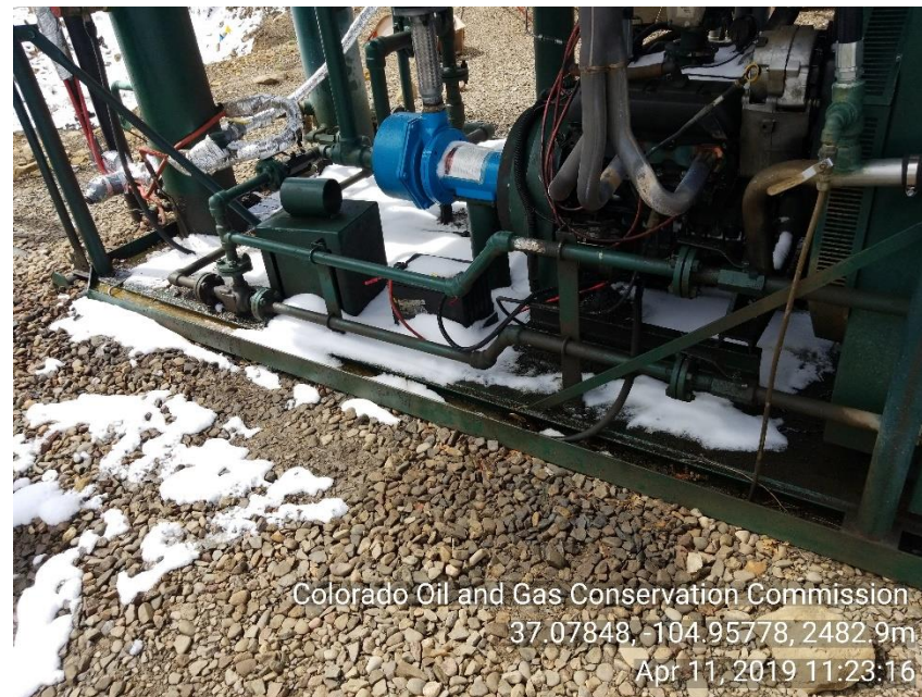
Photo 4 Stained soil around Liquid ring skid.
