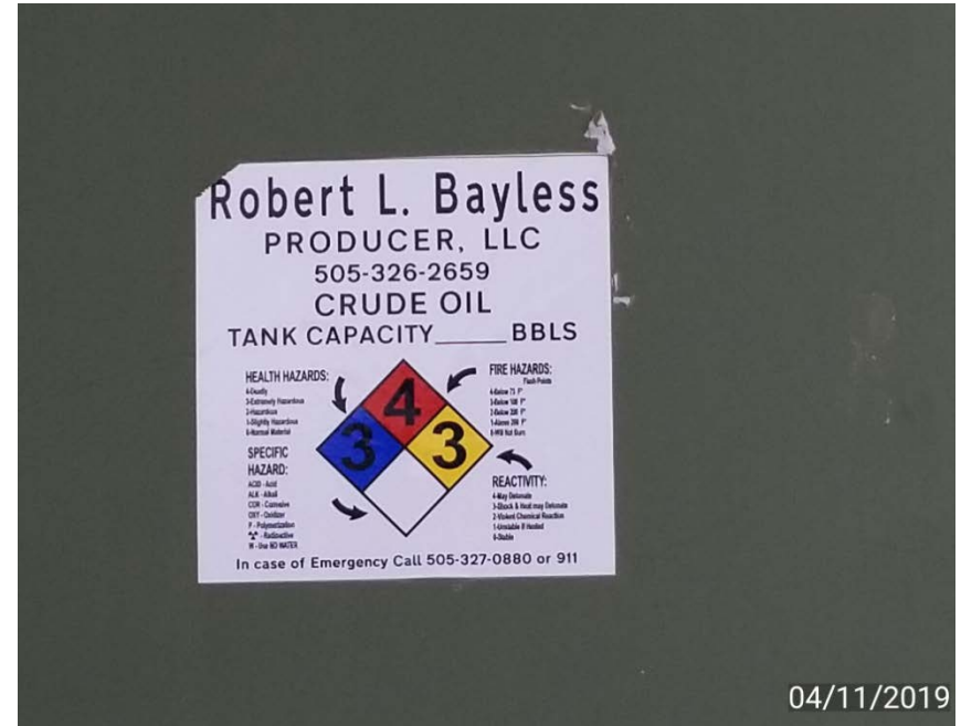
Photo 2. Tank label without capacity volume.
