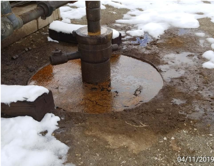
Photo 3. Full well head cellar and surrounding oily waste on ground.
