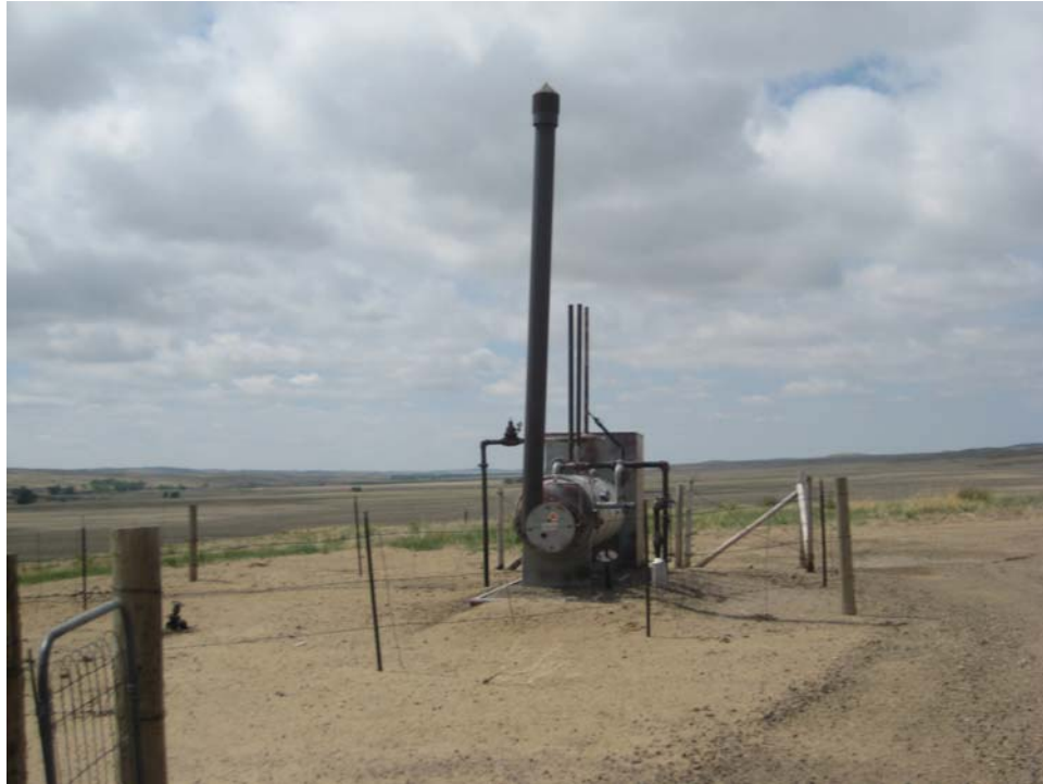
Photo 3. Horizontal separator
