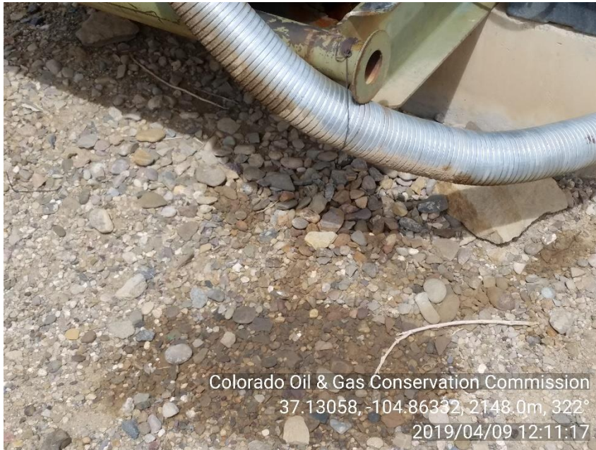
PHOTO 5: APPROXIMATELY 2' BY 2' AREA OF IMPACTED SOIL ON SOUTHEAST CORNER OF ENGINE SKID.
