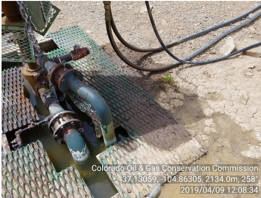
PHOTO 3: APPROXIMATELY 4' BY 2' AREA OF IMPACTED SOIL ON WEST SIDE OF WELLHEAD WITH WHAT APPEARS TO BE HYDRAULIC OIL FROM DRIVEHEAD OR HYDRAULIC HOSED
