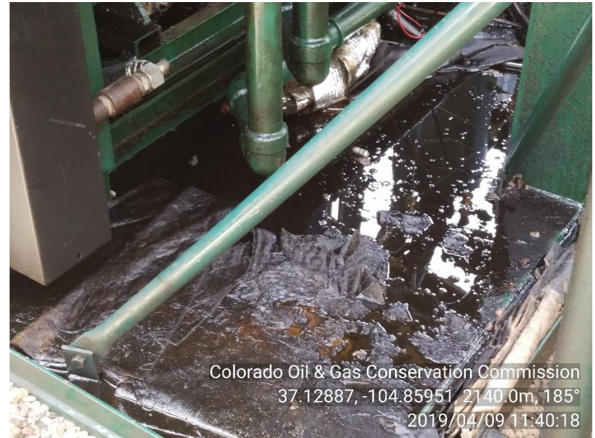
PHOTO 4: COMPRESSOR SKID IS FULL OF OIL AND TRASH CASING SUBSTANTIAL IMPACTED SOIL AROUND SKID. ENTIRE SKID AND ITS COMPONENTS ARE SATURATED WITH OIL.
