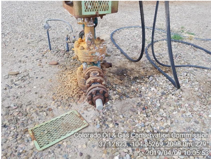
PHOTO 3: IMPACTED SOIL AROUND WELLHEAD A CHALKY RUST COLLARD IMPACTION TO THE LEFT OF WELLHEAD AND AN OILY IMPACTION TO THE RIGHT (WEST) OF WELLHEAD. DRIVEHEAD IS NOT RUNNING AT TIME OF INSPECTION.
