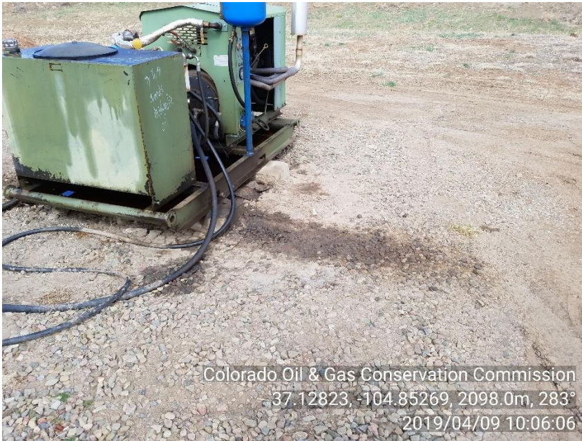
PHOTO 5: IMPACTED SOIL TO NORTH OF SKID AND ALONG HYDRAULIC HOSES LEADING FROM SKID TO WELLHEAD
