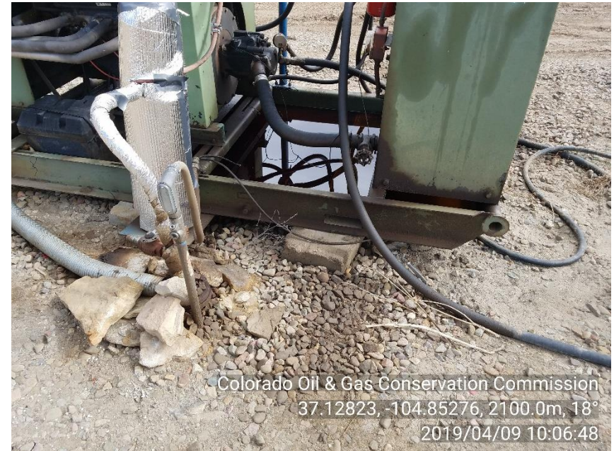
PHOTO 4: ENGINE SKID HAS ROUGHLY 1 TO 1.5" OF OIL. IMPACTED SOIL ON SOUTH SIDE OF ENGINE SKID.
