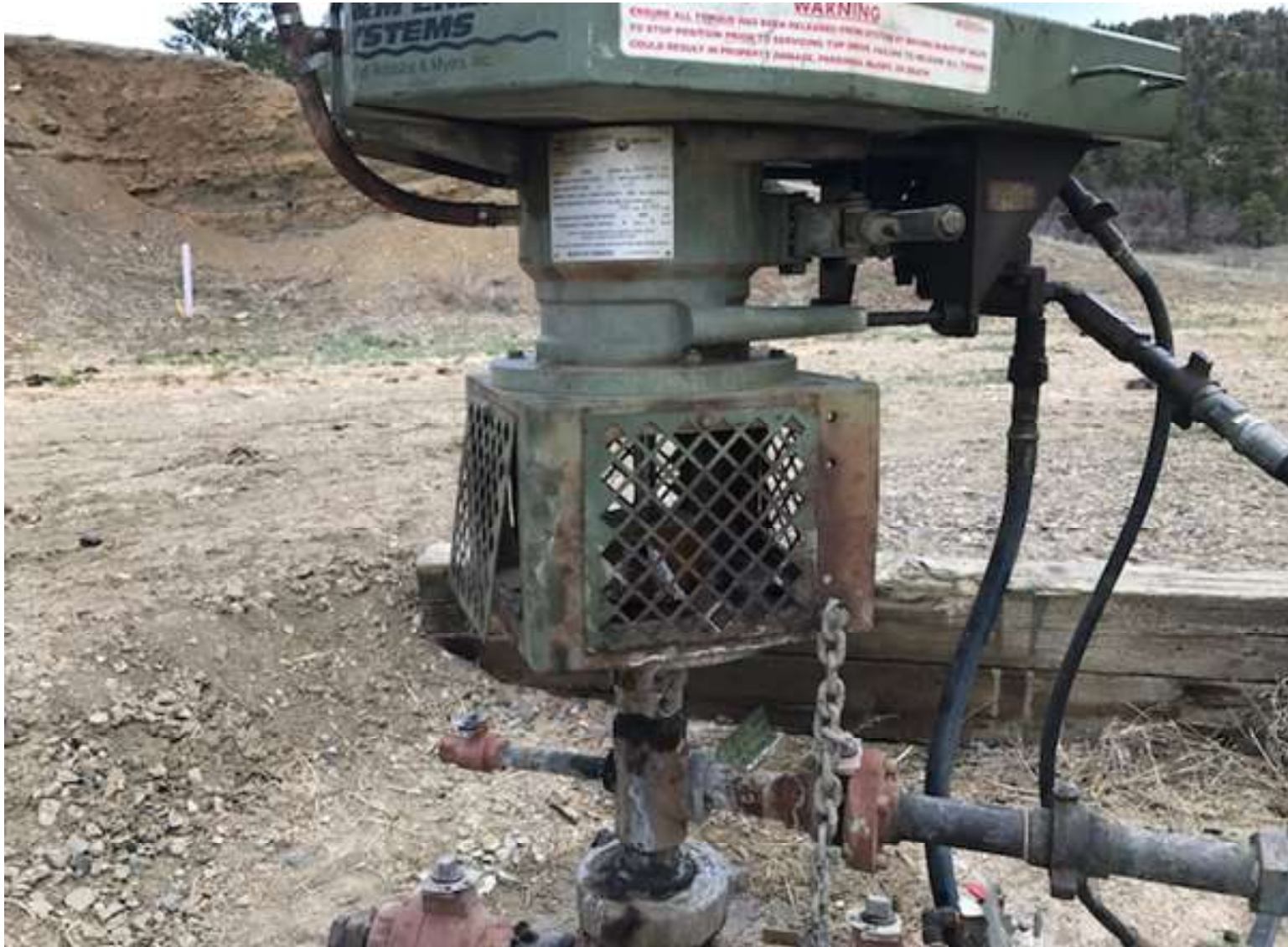
PHOTO 4: THE PACKINGS WERE SECURELY FASTENED TO STOP THE LEAK AND ENSURE GOOD MECHANICAL CONDITION.
