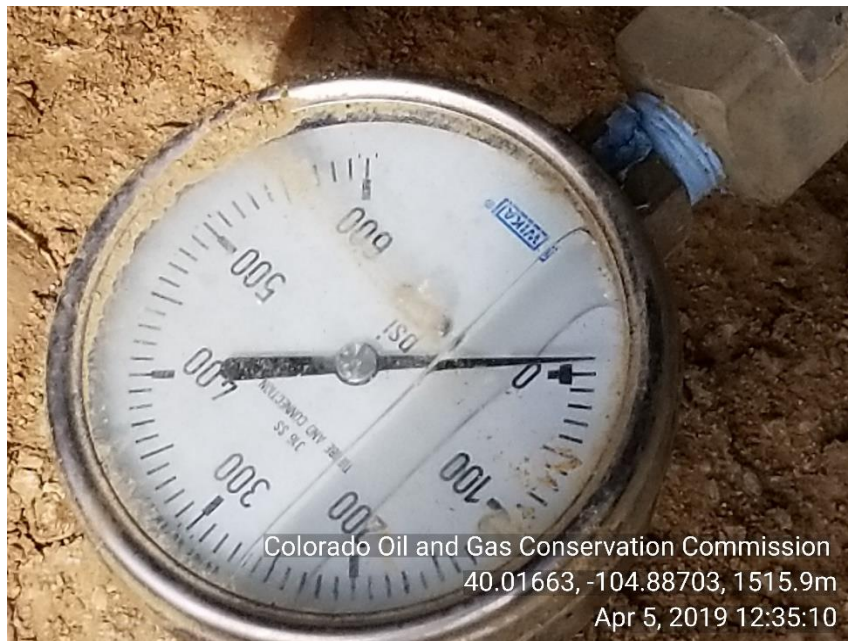
Photo 3 casing pressure Opsig
