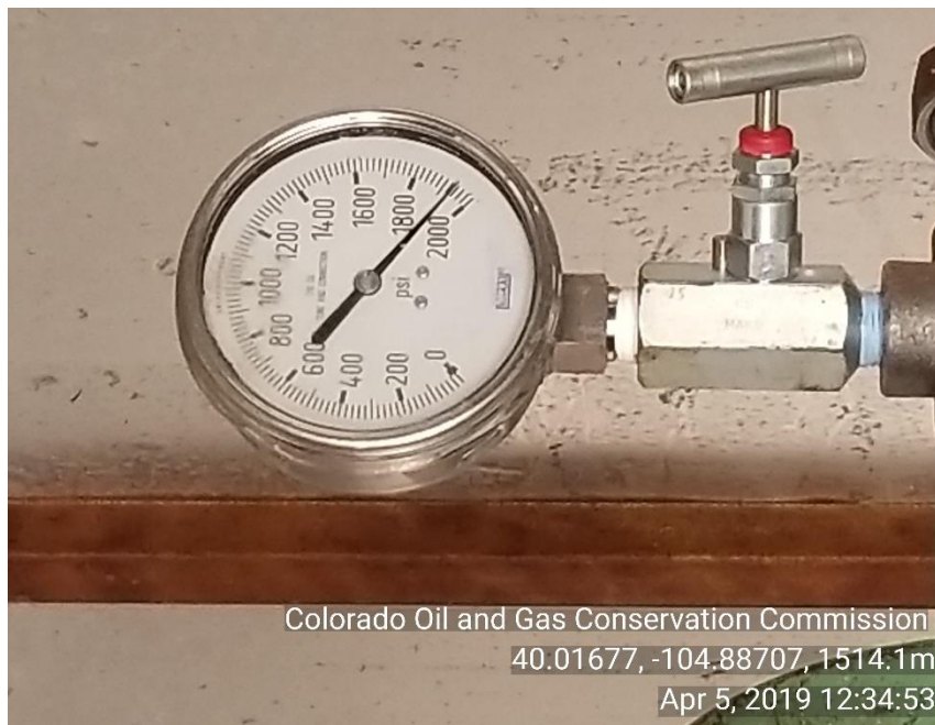
Photo 1 Tubing pressure 1900psig
