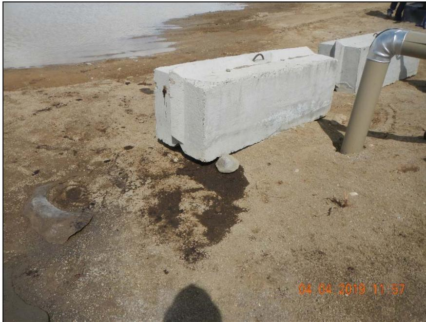
**Photo 21. Non-reportable spill, stained soil outside containment.**
