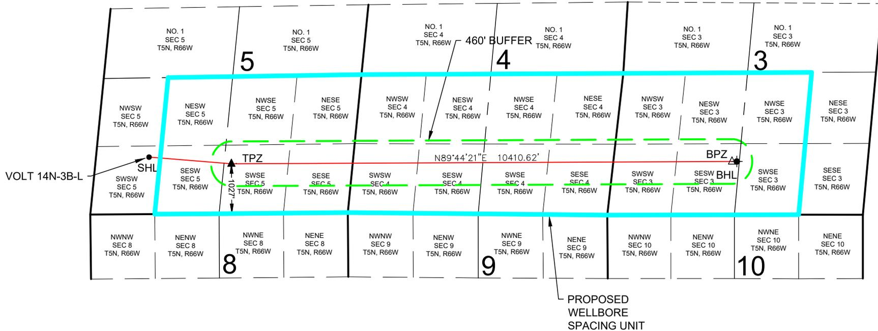
**VOLT 14N-3B-L WELL TO BE LOCATED 1175' FSL AND 1087' FWL, SEC 5, T5N, R66W**
