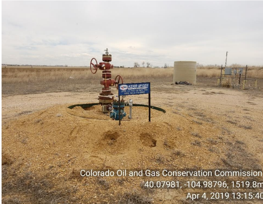
Photo 1 WH piping from injection line to WH has been removed no gauge on tubing on top of WH
