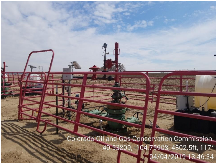
Photo 7 – 34R-203 Wellhead Sign is missing
