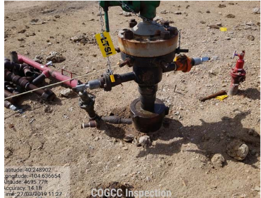
Photo 4 – Wellhead not cut and capped. Localized stained soil and fluid observed at wellhead.
