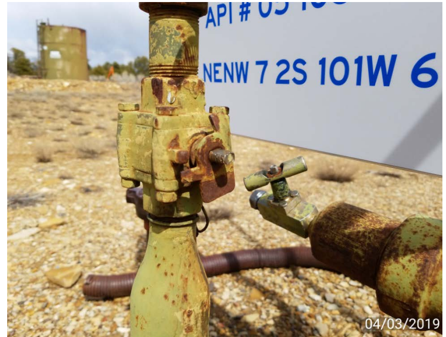
Photo 3. Well head - casing valve closed.
