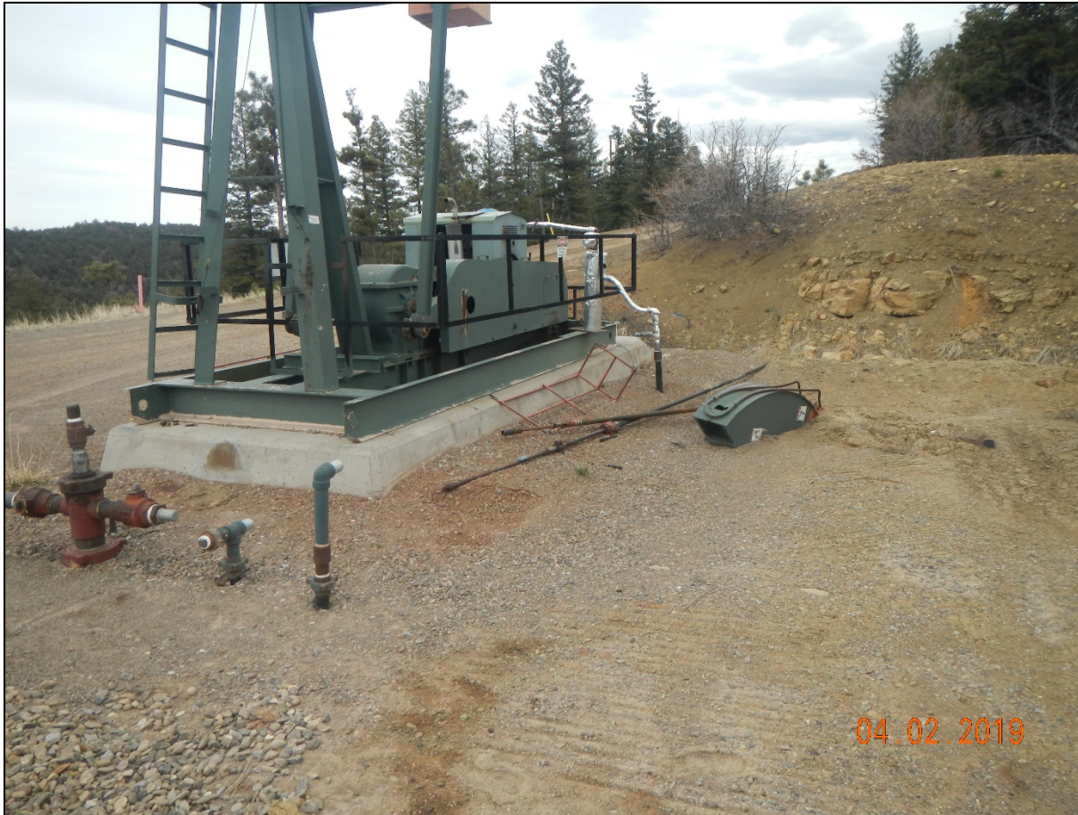
Photo 2. It does not appear that risers are LOTO and unused equipment still remains.
