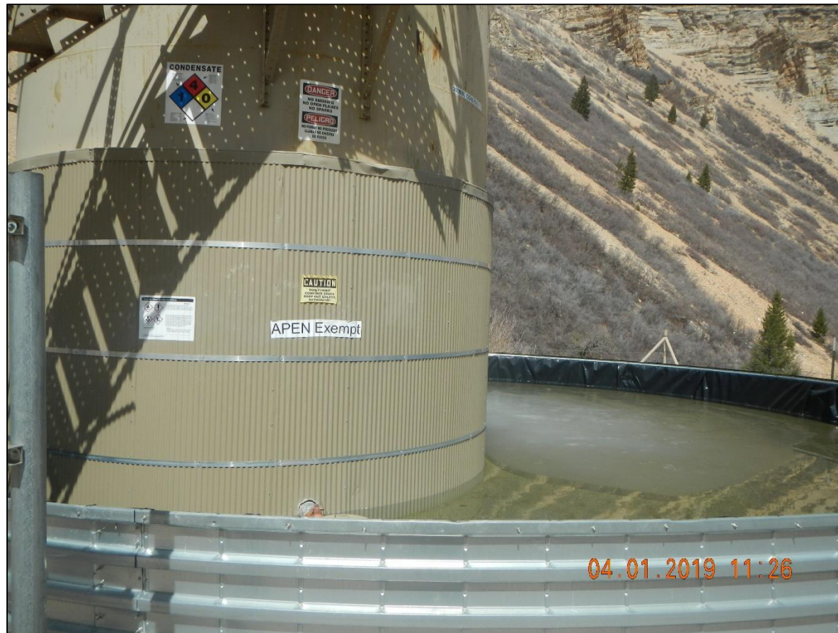
Accumulation of fuilid inside of containment.
