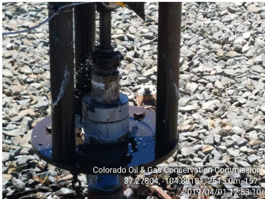
PHOTO 3: PACKING IS SPRAYING PRODUCED WATER OUT ON LOCATION.
