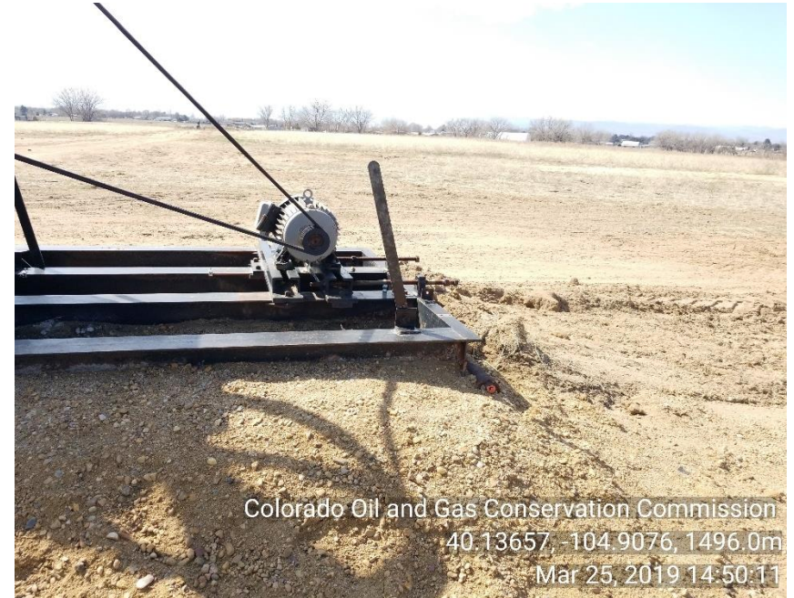
Photo 2 electric power has been removed
