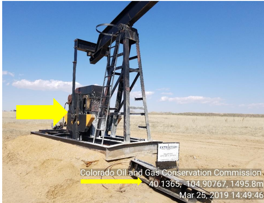
Photo 1 Well is P&A unused equipment (PU horses head)
